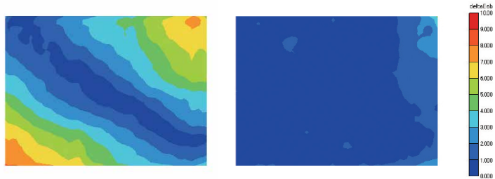
DIGITAL UNIFORMITY CONTROL Before Digital Uniformity Control is applied (Left) After Digital Uniformity Control is applied (Right)
